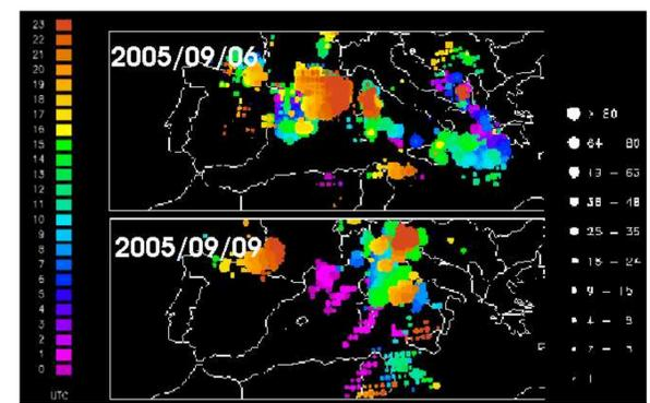
FIGURE 4: Lightning activity recorded by the UK Met Office ATD lightning network in Europe ([www.torro.org.uk/sfinfo.htm](http://www.torro.org.uk/sfinfo.htm)).
