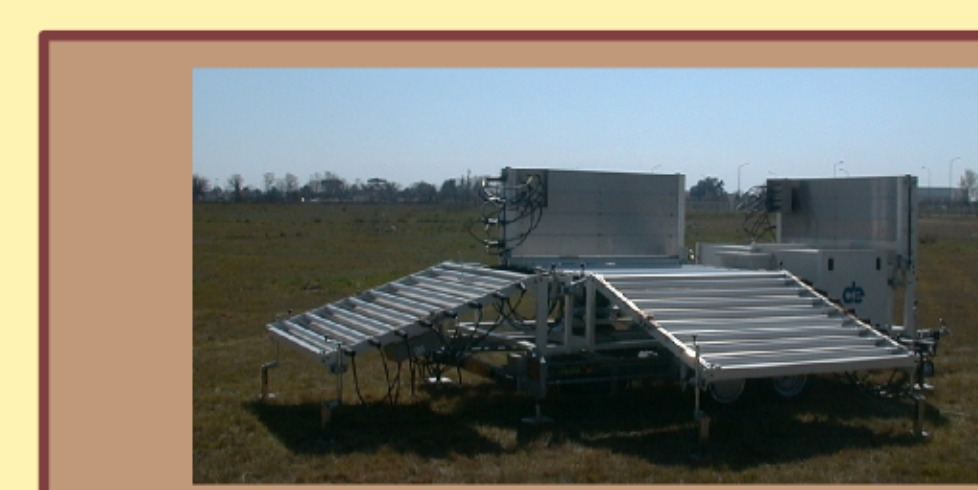
Degreane PCL 1300 mobile UHF wind profiler (1274 MHz)
